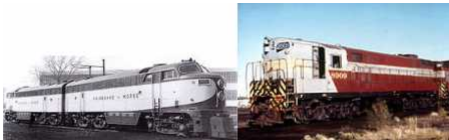
FM 2400 HP CPA24-5 and Trainmaster H24-66, 2400HP Locomotives, both using opposed piston engines.
